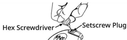
3. When a single-receptacle generator and single-pin lead is used, insert the lead connector pin fully into the generator header. To allow escape of the back pressure created by insertion, leave the tip of the hex screwdriver in the slit in the setscrew plug.
