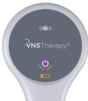
Figure 7. Low Battery Indicator
